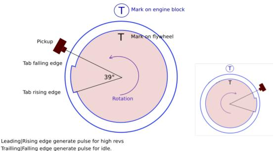
Trailling|Falling edge generate pulse for idle.
