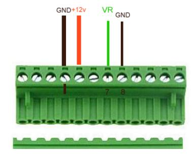
To avoid ElectroMagnetic Interference (EMI) it's safer to connect the pickup sensor through a shielded cable. Shield grounded on ignition box side only.
