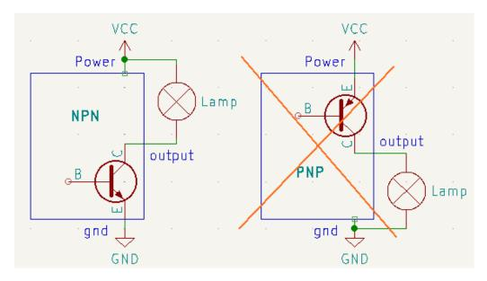
NPN Proximity Sensor Output is normally HIGH when nothing is near it. NPN Proximity Sensor Output goes LOW when metal object is near it.
