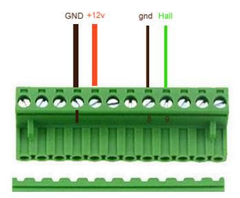
When Hall sensor is connected to pin 9 = "Pickup Type" must be set to [2] in Setup
