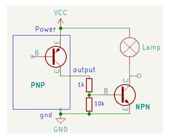
*Tip: A PNP type can be used if there is an external NPN transistor to reverse the signal:*
