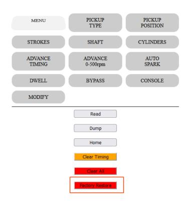
Timing, Pickup position, polarity, shaft, dwell etc are set to default values.
