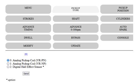
Select the type of pickup attached to the Ignition box:
