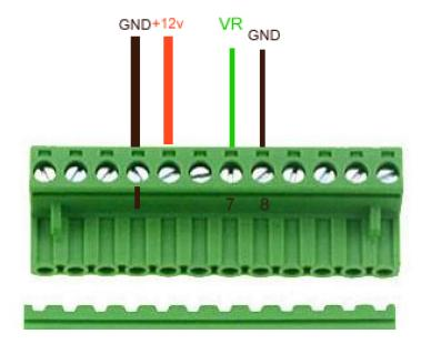
To avoid ElectroMagnetic Interference (EMI) it's safer to connect the pickup sensor through a shielded cable. Shield grounded on ignition box side only. Twisted pair is better.
