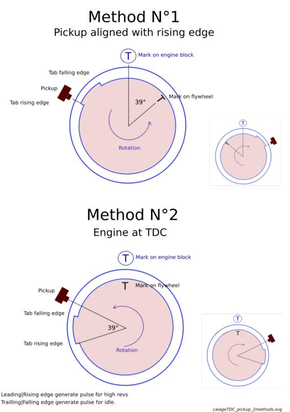
This view above represents the respective positions of the rotor and the pickup as we would see them if the engine cover were transparent.
