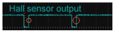
The rising edge of the signal appear when the magnet <u>leaves</u> the hall sensor, therefore when the hall sensor is aligned with the **falling edge of the magnet**.
