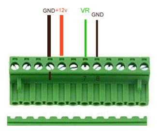
The pickup coil MUST be connected in order to send a POSITIVE PULSE FIRST:
