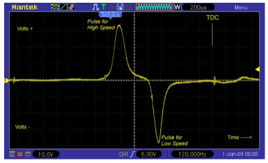
If the first pulse is Negative then the timing will be completely off (spark AFTER TDC).
