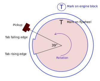
Leading|Rising edge generate pulse for high revs Trailling|Falling edge generate pulse for idle.
