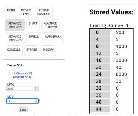
RPM can be entered with a 100rpm step but RPM will be measured with **1rpm** precision.
