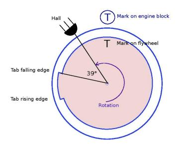
A) Remove the sparkplug, find the TDC position with a *dial indicator gauge* or a *caliper rule*:
