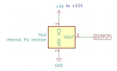
Hall sensors require a +5v to +12vdc supply voltage.
