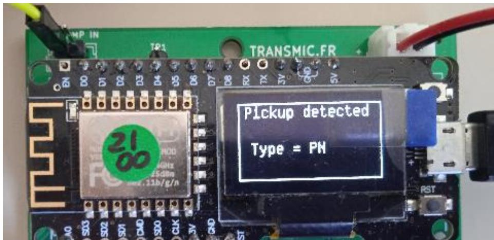
If *Pickup Type* is already set to **NP** or **PN**, "Start Engine" disappear after 2 seconds and ITM goes into RUN mode
