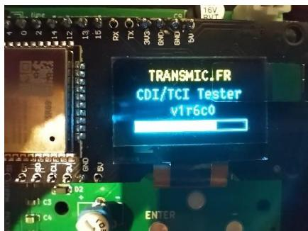
To launch the SETUP mode, touch "**ENTER**" button, otherwise wait **10 seconds** until it goes into RUN mode:
