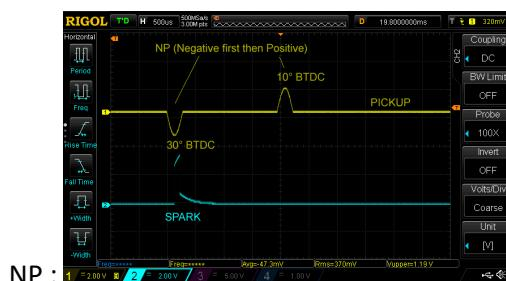
It's important to understand that calculation starts from the first pickup pulse.
