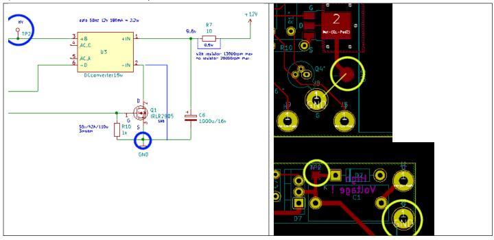
Power on the unit. Check if around 300Vdc between GND and TP2
