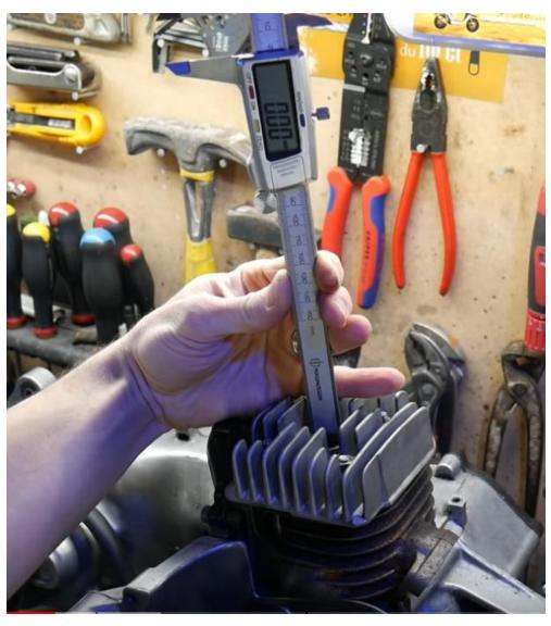
B) Align the pickup with the beginning of the magnet on the rotor and measure the travel of the piston with the caliper rule:
