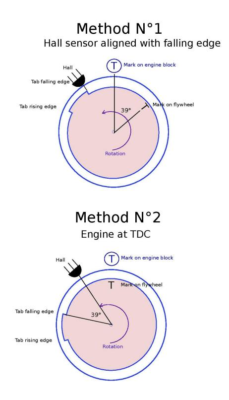
A) Remove the sparkplug, find the TDC position with a *dial indicator gauge* or a *caliper rule*:
