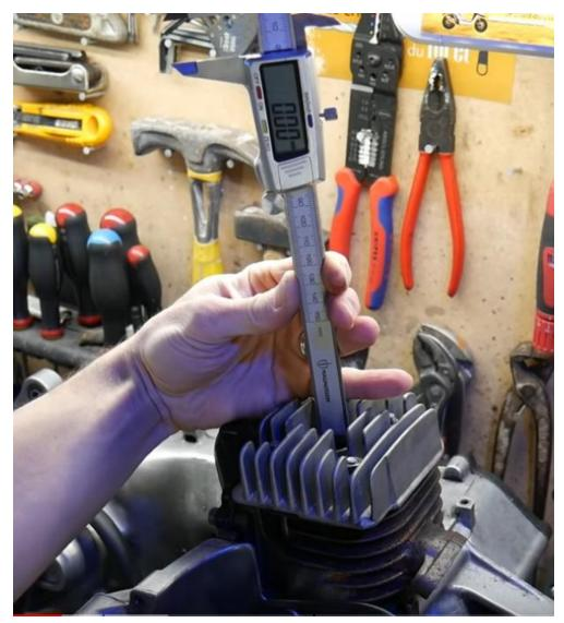
B) Align the pickup with the beginning of the magnet on the rotor and measure the travel of the piston with the caliper rule:
