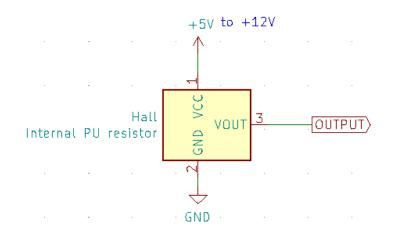
Hall sensors require a +5v to +12vdc supply voltage. See datasheet
