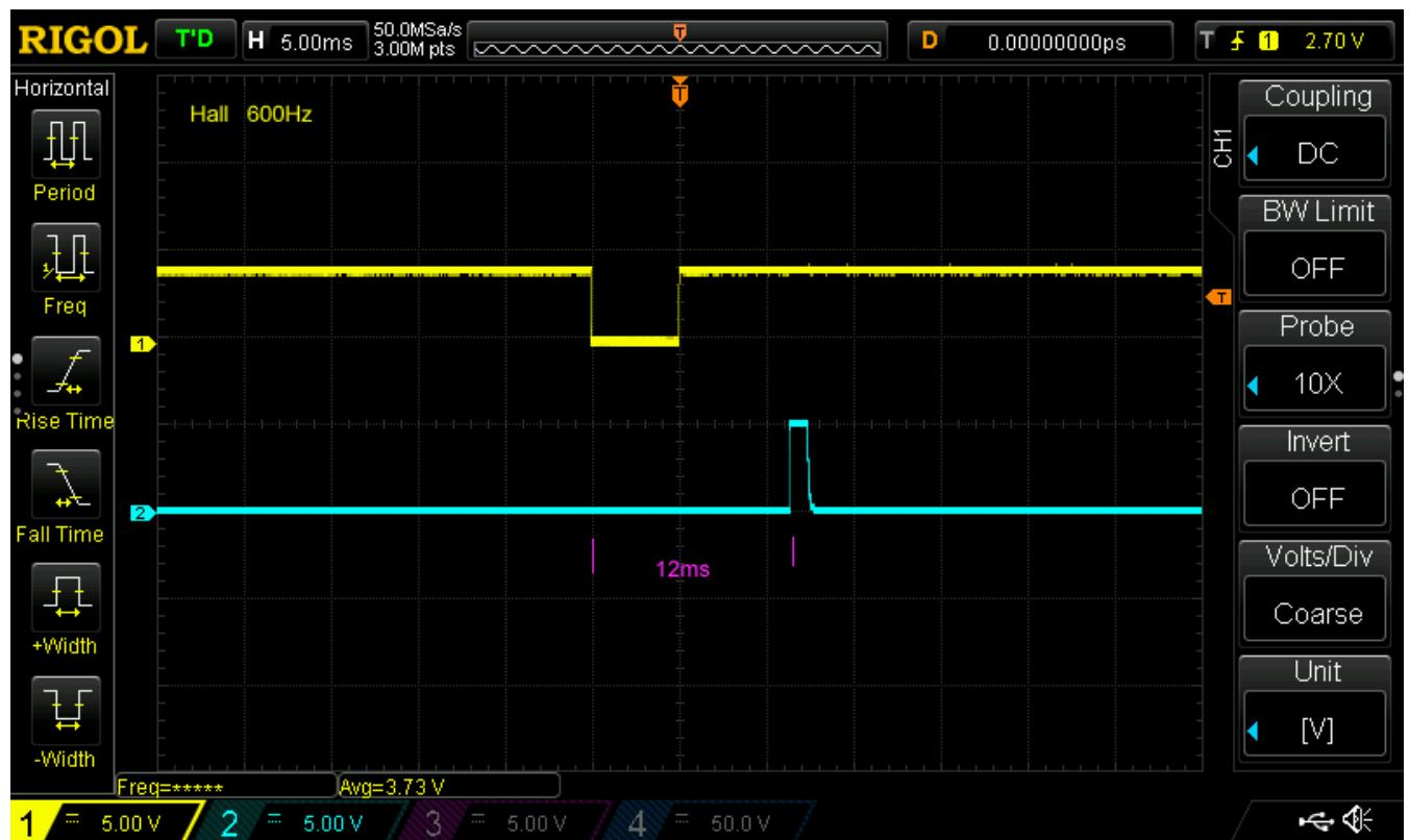
The falling edge of the signal appear when the magnet reaches the hall sensor, therefore when the hall sensor is aligned with the **rising edge of the magnet**.
