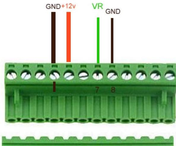
*To avoid ElectroMagnetic Interference (EMI) it's safer to connect the pickup sensor through a shielded cable. Shield grounded on CDI side only.*
