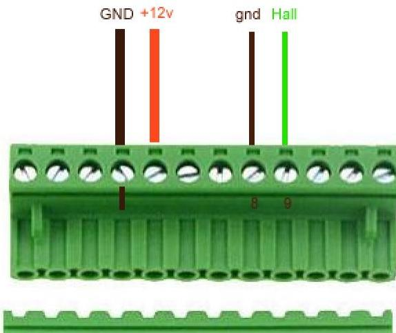
When a Hall sensor is connected to pin 9, then "Pickup Type" must be set to **2** during Setup.
