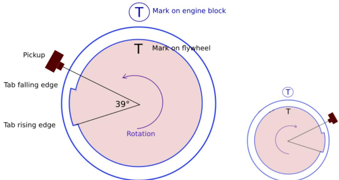
Leading|Rising edge generate pulse for high revs
