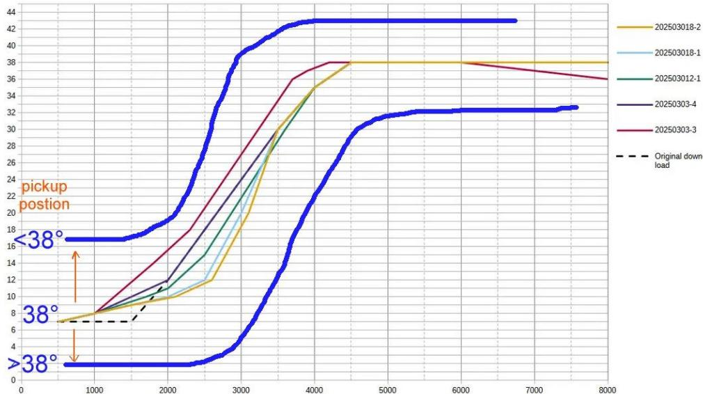
2) Pickup position **MUST** always be larger than the maximum advance timing.
