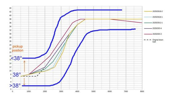
2) Pickup position MUST always be larger than the maximum advance timing.
