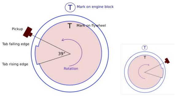
Leading|Rising edge generate pulse for high revs Trailling|Falling edge generate pulse for idle.
