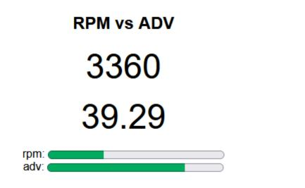
Display appears ONLY when the engine is running.
