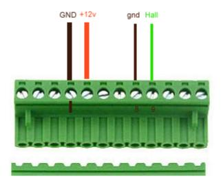
When Hall sensor is connected to pin<sup>9</sup> = "<u>Pickup Type</u>" must be set to [2] in Setup
