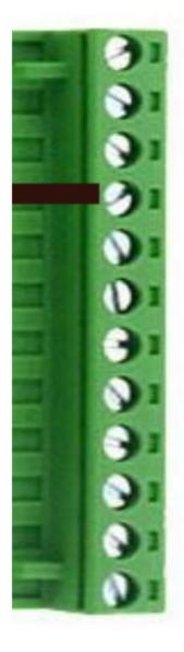
To ignition coil 1 output High Voltage from Charging Coil 2 input High Voltage from Charging Coil 3 input ground frame (=minus from battery) 4 input +12Vdc from battery 5 input 6 input Kill switch 7 input Analog Pickup 8 Pickup or Hall Sensor Ground input 9 input Digital Hall Effect Sensor \* 10 input If second analog Pickup for Low RPM 11 output Tachometer \* 12 input Curve Selection \*
