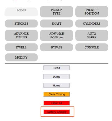
Timing, Pickup position, polarity, shaft, dwell etc are set to default values. (Payed Options are kept)
