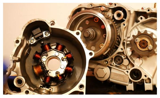
In this example below the pickup/sensor is set at 39° BTDC
