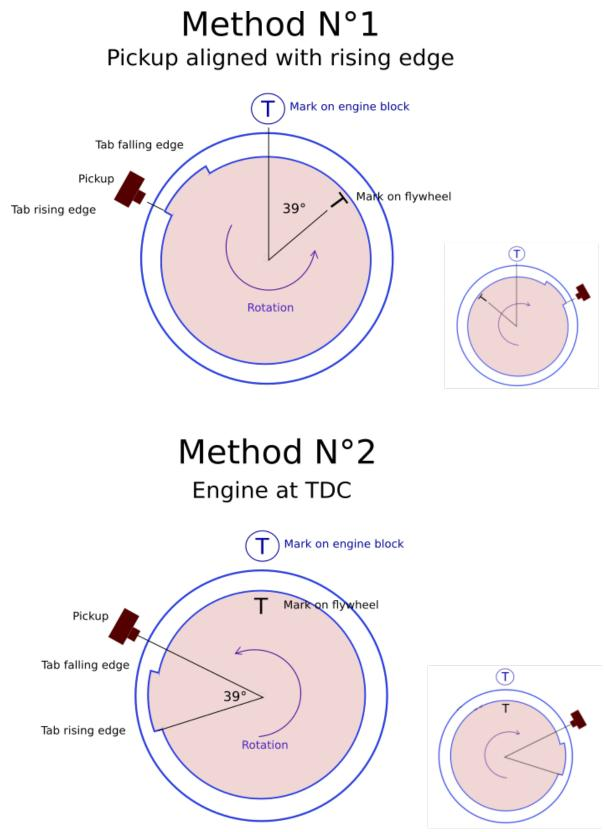
Leading|Rising edge generate pulse for high revs Trailling|Falling edge generate pulse for idle.
