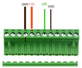
To avoid ElectroMagnetic Interference (EMI) it's safer to connect the pickup sensor through a shielded cable. Shield grounded on CDI side only. Twisted pair is better.
