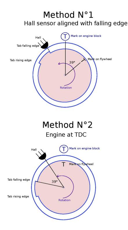
A) Remove the sparkplug, find the TDC position with a *dial indicator gauge* or a *caliper rule*:
