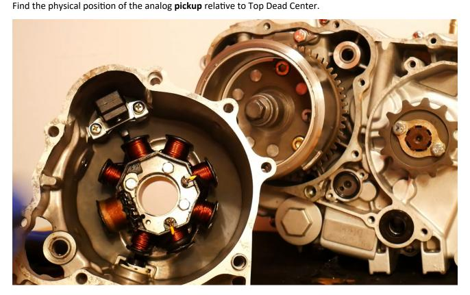
In this example below the pickup/sensor is set at 39° BTDC
