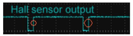
You can even connect an **Optical Sensor** as long as it puts out a CLEAN square signal similar to the one above.
